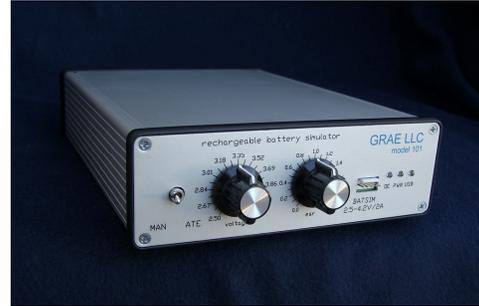
It emulates a single Lithium-Ion cell or pack of up to 2000maHr capability. The characteristics of a real-world cell such as battery terminal voltage, equivalent series resistance (ESR) and pulsed-load voltage decay are implemented in circuitry and software. The output is two quadrants in operation. It is possible to source or sink current to the device under test (DUT). Thus it can be “re-charged” like a battery.
